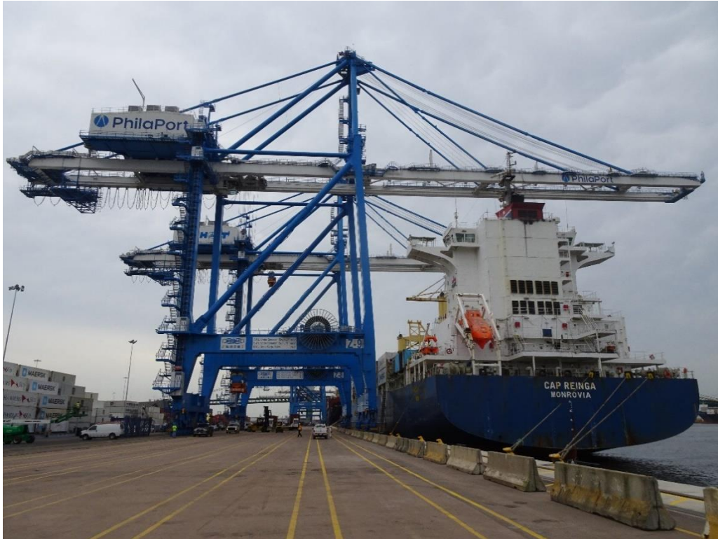
Pictured: PAMT ‘new’ STS manufactured by foreign supplier and equipped with MV Cable Reel System.
